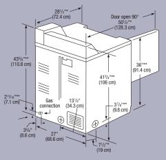
\* Includes  ${\ensuremath{\rlap/}\!\!\!\!{}^{\prime\prime}}$  (1.9 cm) for hinge on back of dryer.
